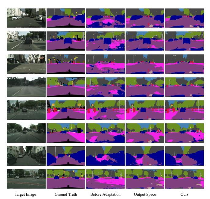
Figure 3. Example results of adapted segmentation for the SYNTHIA-to-Cityscapes setting. For each target image, we show results before adaptation, output space adaptation [4], and the proposed method.
