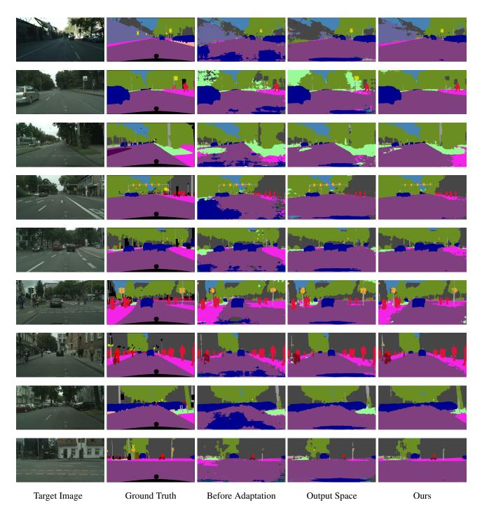
Figure 1. Example results of adapted segmentation for the GTA5-to-Cityscapes setting. For each target image, we show results before adaptation, output space adaptation [4], and the proposed method.
